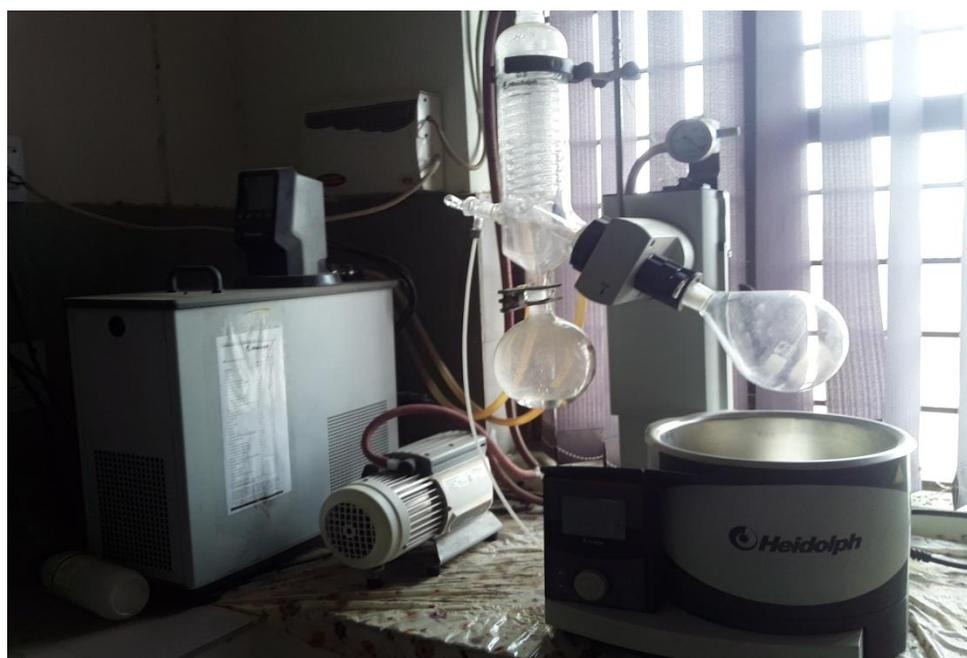
Figure 2.3 : Rotary evaporator (Heidolph G3, Germany)
