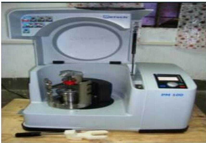
**Figure 2.4: RETSCH Planetary Ball Mill**
