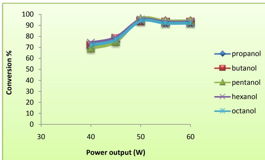
**Figure 3.10: Variation of conversion (%) of alcohols over catalyst with power output.**
