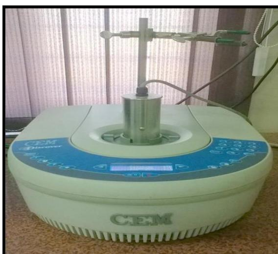
Figure 2.1: CEM Focused Microwave<sup>TM</sup> Synthesis System (Discover Model)
